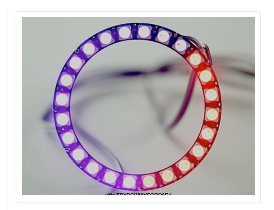
This project (http://www.insentricity.com/a.cl/268/controlling-ws2812-rgb-ledsfrom-the-esp32) uses the RMT peripheral of the ESP32 to control WS2812 RGB LEDs.
