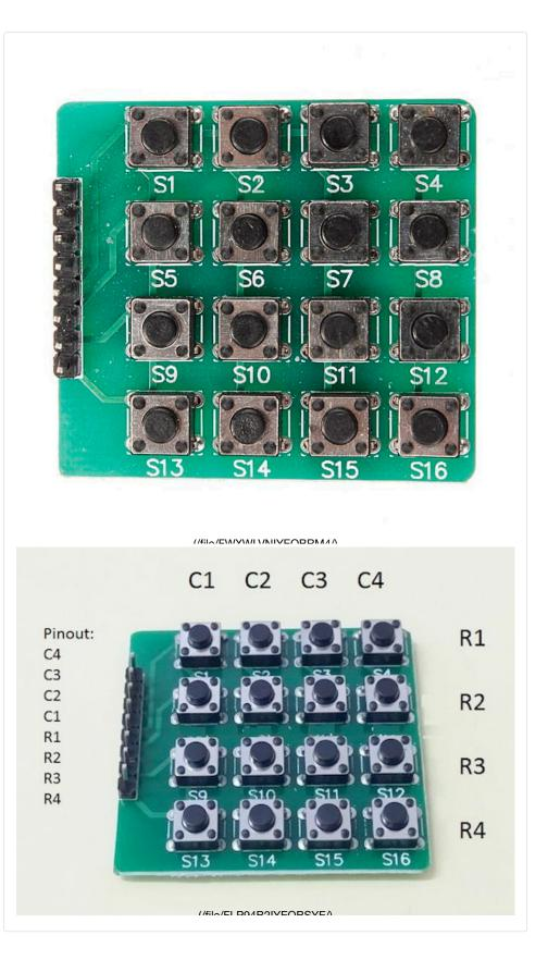
The Arduino Playground Matrix Keypad Tutorial (http://playground.arduino.cc/Main/KeypadTutorial) is a good starting point for working with this type of keypad. Suggested applications:
