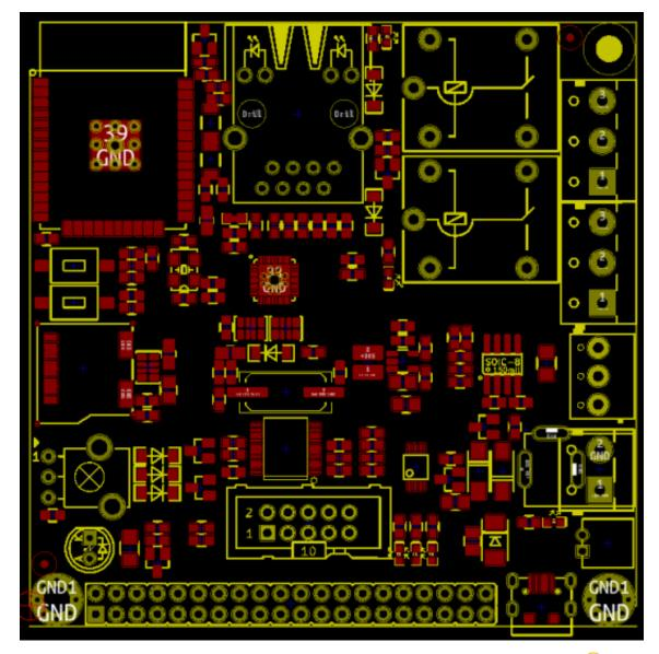
ESP32-EVB revision A was made quick and has too many errors  $\bigcirc$  some were due to the non very clear documentation, like that we assumed that all ports could have internal pull-ups but when we try to write the software we found that the GPIOs we used for the buttons has no such. Other were done by our engineer negligence.
